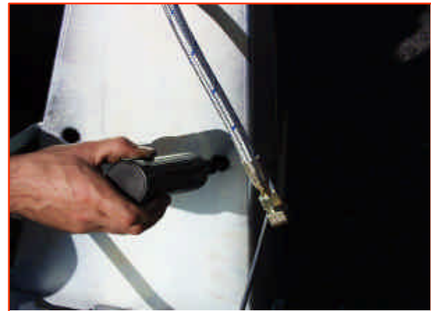
Fig 9: Grease pump at two grease points after intensive use.
