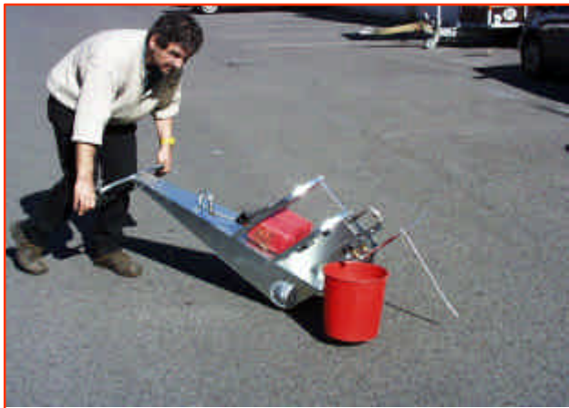
Fig 8: To clean system pull back the spray cart with pulled grip to pump back primer into can. Afterwards clean system with solvent.
