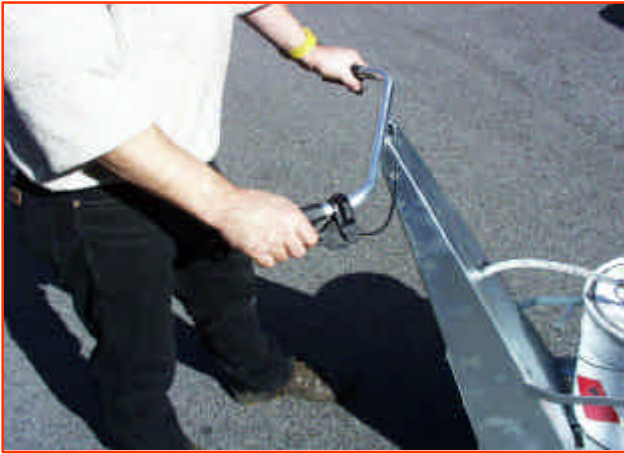
Fig 6: To spray pull handle grip. Releasing grip stops pump.
